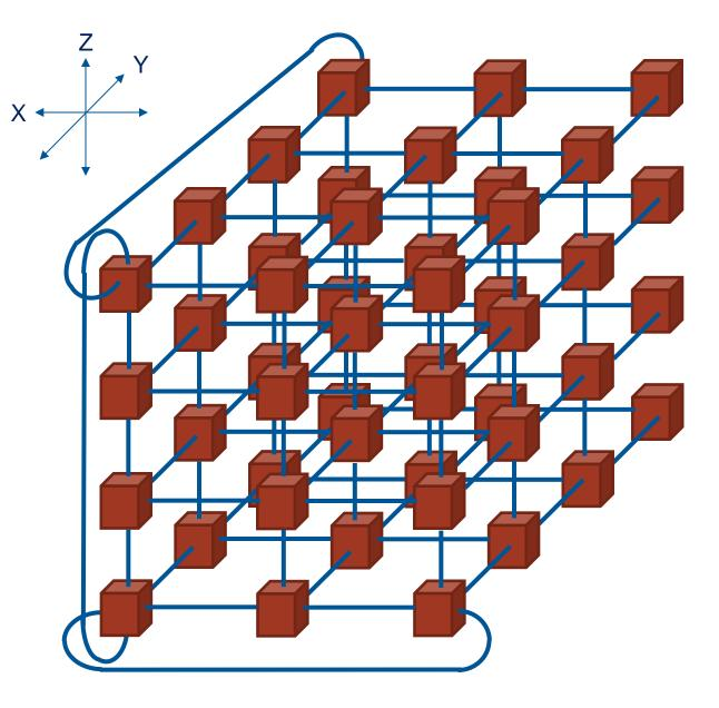
The Cray XE6 connects nodes together in a 3D Torus,
